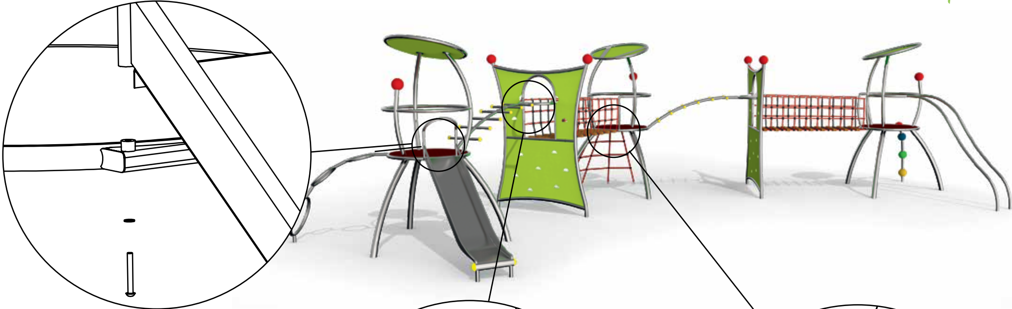
Diagram 6a: Attachment part slide
